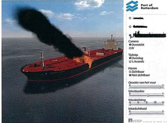
In the Incident Configurator tool that VSTEP made for the Port of Rotterdam authorities, an instructor can configure an incident to his preference. He can choose from three ship types, set the location (inside the harbour or on open sea), and set some weather conditions like wind direction and force. Students subsequently experience the incident from a viewpoint of an incident response ship. In a classroom, they discuss the best way of attacking the fire.
